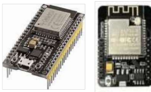
Gambar 2.1 Modul ESP32 Sumber: Setiawan,agung. (2012)
