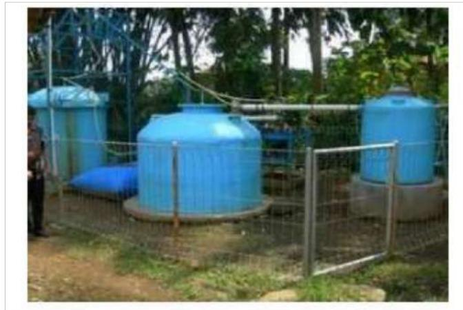
**Gambar 2.4 *Digester Fiber Glass***
