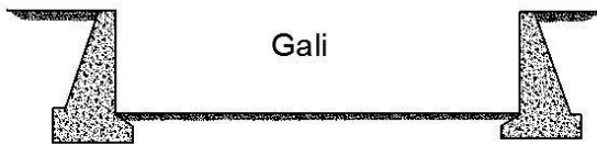
(c) Penurunan Jalan/Rel
